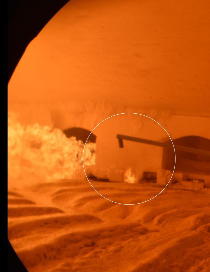
Hot Face Ceramic Welding Breast Wall Tuck Line All ceramic welding materials used by Fuse Tech are mixed in house, by Fuse Tech employees guaranteeing the highest quality materials are utilized in our process.
