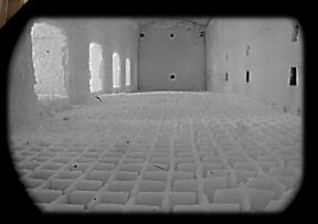
Using a water-cooled periscope our high-temperature imaging system provides you with valuable insight into what is going on in your kiln or furnace, enabling you to view areas or actions that may not be visible through normal line of sight.
